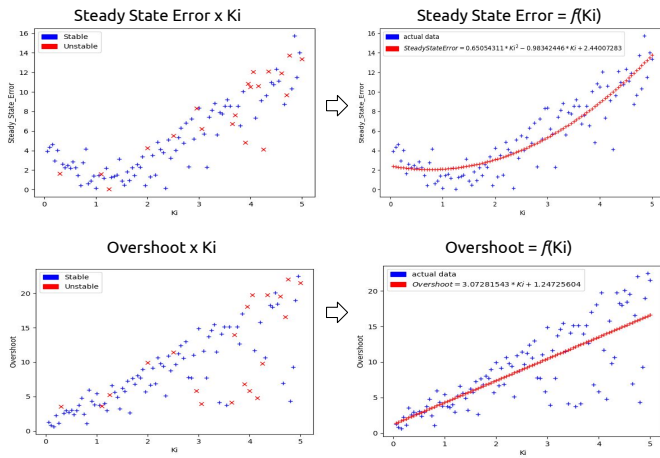
Figure 7: Model learning by curve fitting the behavior of the strategy enactor.
